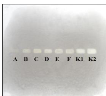
Figure 4. HPTLC-tyrosinase assay, extracts (200 µg) and kojic acid, (A, kumquat (b) extract; B, kumquat (a) extract; C, limequat (b) extract; D, limequat (a) extract; E, Mexican lime (b) extract; F, Mexican lime (a) extract; K1, kojic acid 5 µg; K2 kojic acid 20 µg; (b), extract obtained from unheated fruit powder; (a), extract obtained from heat-treated fruit powder).
