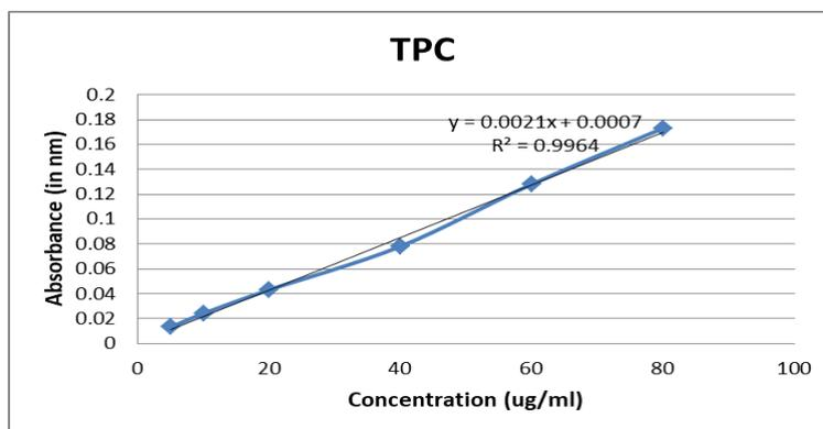
Figure 2. Calibration Curve of Gallic acid (Standard)
