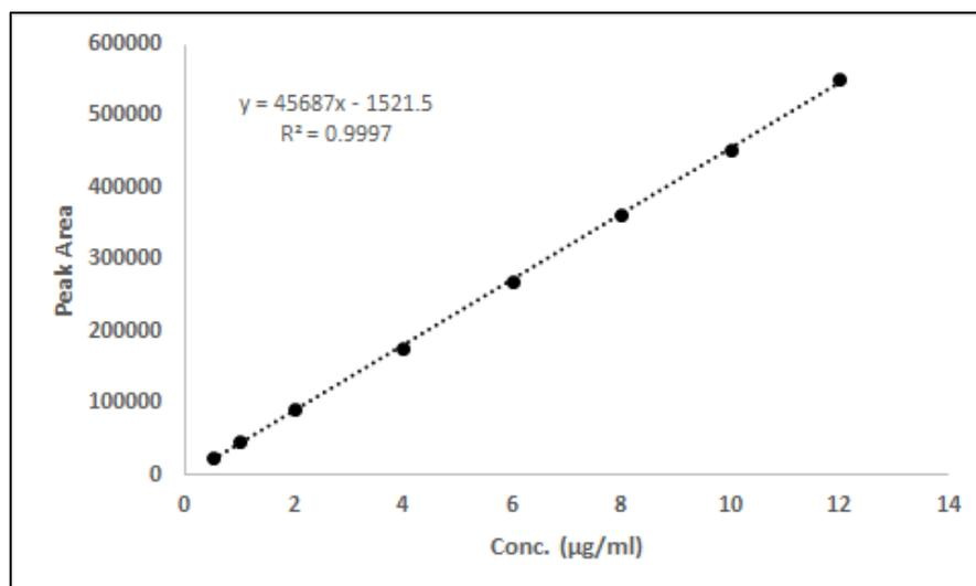
**Figure 3.** Calibration curve of ketoconazole used RP-HPLC method with mobile phase used acetonitrile: water with TEA 0.15% pH 3.3 (50:50)
