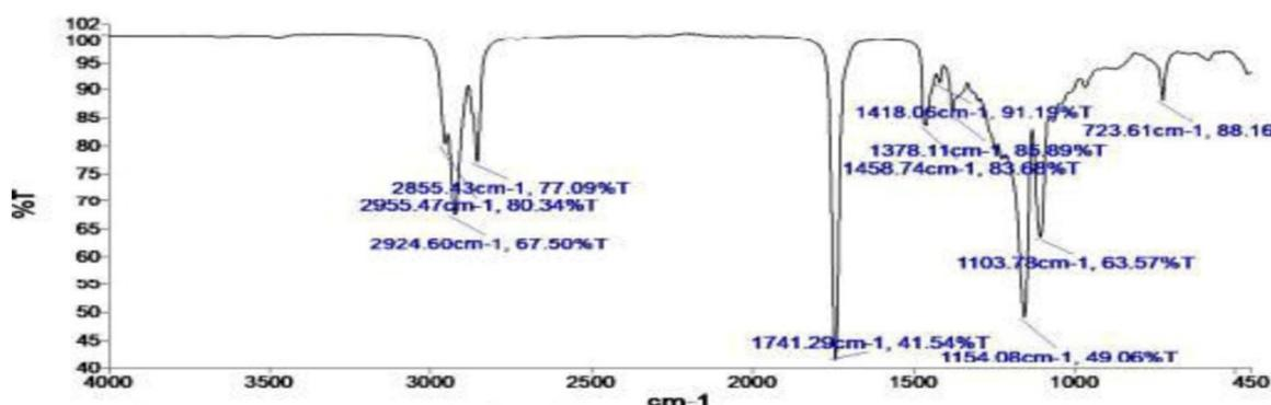
Figure 2. FTIR of pure drug ascorbic acid
