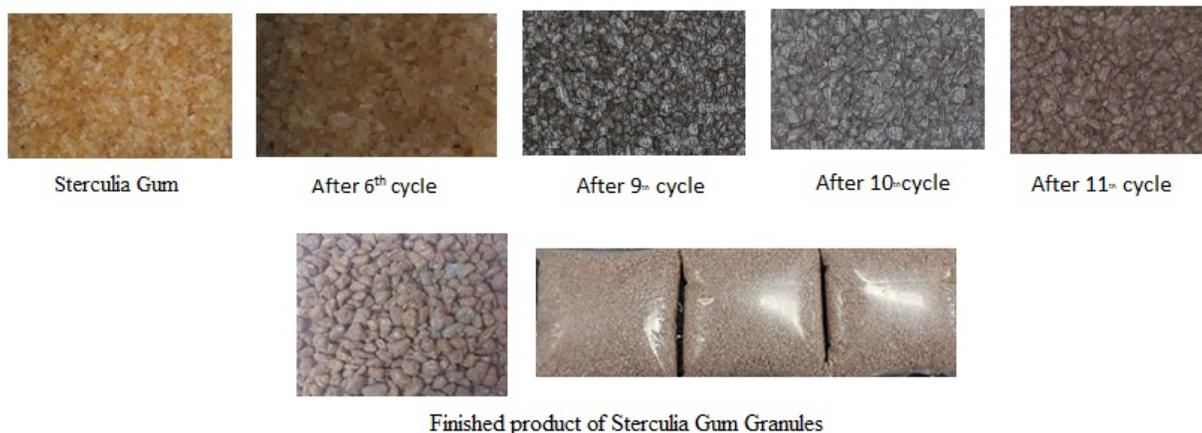
Figure 2. Raw Sterculia Granules (standard), Appearance of granules after 6<sup>th</sup> cycle, 9<sup>th</sup> cycle, 10<sup>th</sup> cycle and 11<sup>th</sup> cycle of coating, Finished product of oral laxative Sterculia Gum Granules.
