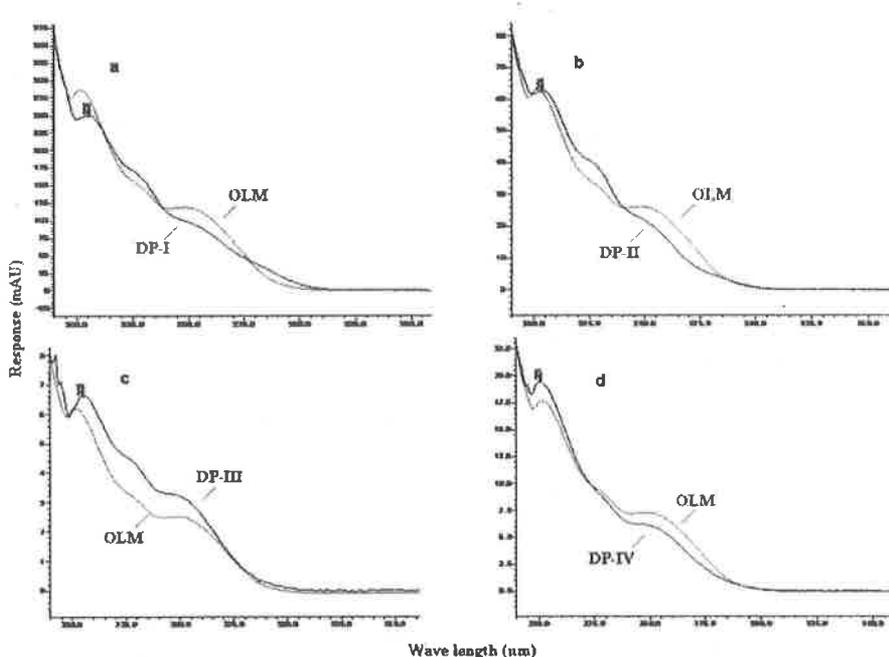
**Figure 3.** Comparative UV spectra between olmesartan medoxomil (OLM) and degradation product (DP-I) (a), DP-II (b), DP-III (c), DP-IV (d). Lack of UV absorption maximum at 260 nm characteristic of ester moiety in both degradation product DP-I and II.
