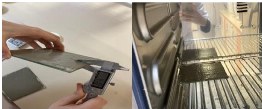
Figure 4. Application of 0.2 mm thick mask on glass plate and determination of drying time ( 37^\circ\text{C} -oven, n=3)
