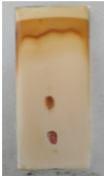
Figure 2. The photograph of chromatograms representing the resolution of enantiomers of ( RS )-KET using FRV as chiral selector in stationary phase. Chromatographic conditions: mobile phase: ACN-MeOH-TEA (6:2:2, pH 9); development time, 10 min; temperature, 25±2 °C, chiral selector FRV in stationary phase, pH 5.0. The spots were visualized in iodine vapor.
