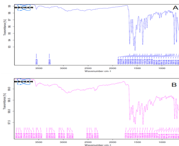
Figure 2. FTIR Spectra of (A) lisinopril (B) lisinopril ion pair
