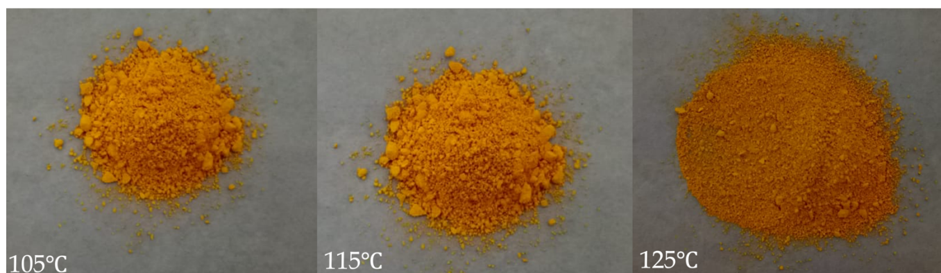
Figure 1. Spray Drying powder of solid dispersion at varying temperatures
