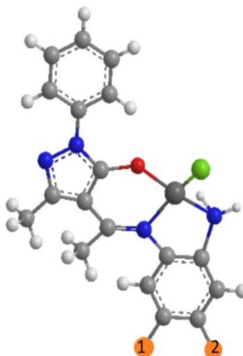
**Figure 5.** Structure of Schiff base compounds: complex A [Pt(SHB247)Cl] (1 and 2: H), complex b [Pt(SHB245)Cl] (1: CH<sub>3</sub> and 2:H) and complex c [Pt(SHB246)Cl] (1 and 2 :CH<sub>3</sub>).
