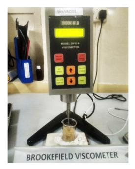
Figure 6: Brookefield viscometer
