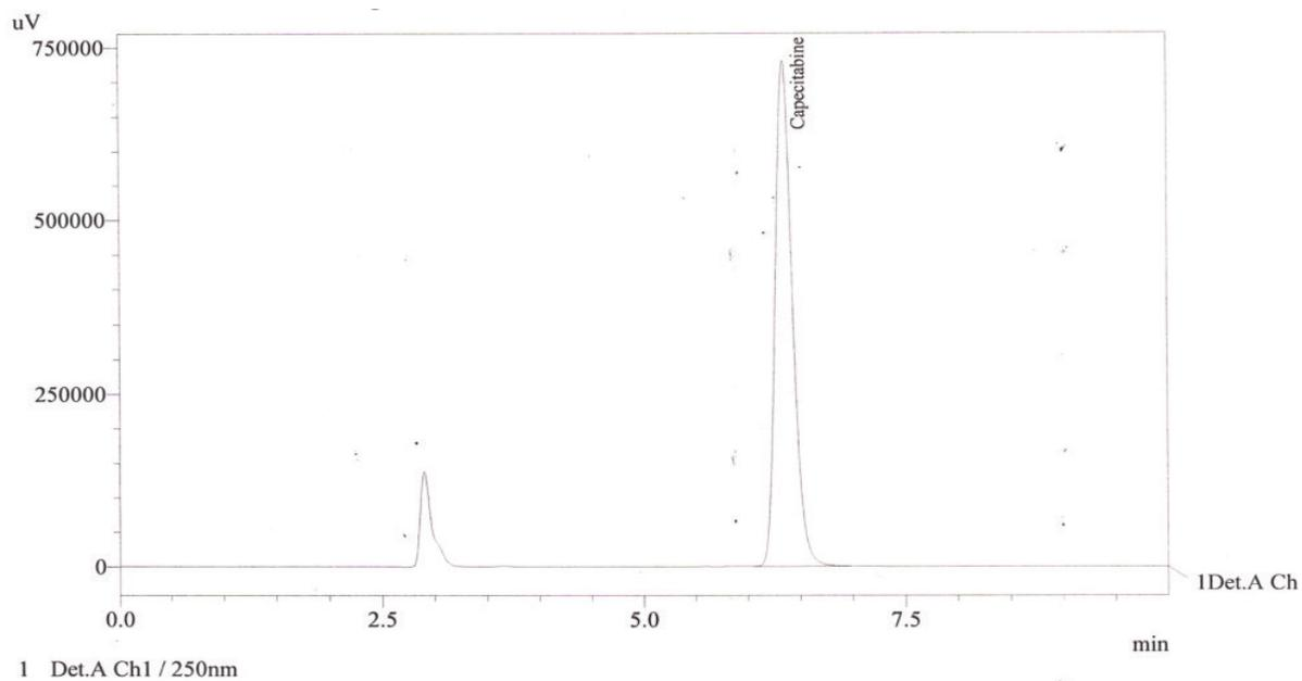
**Figure 4.** Chromatogram for specificity in 0.1M NaOH
