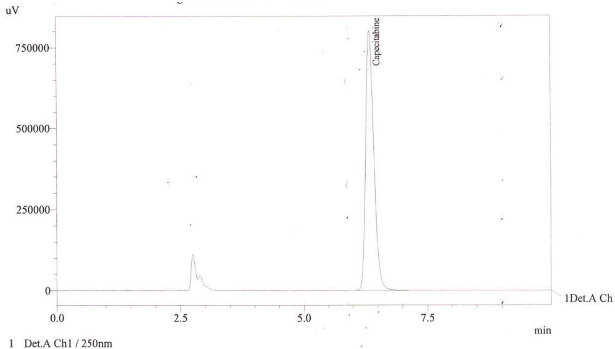
**Figure 5.** Chromatogram for specificity in 10% H<sub>2</sub>O<sub>2</sub>
