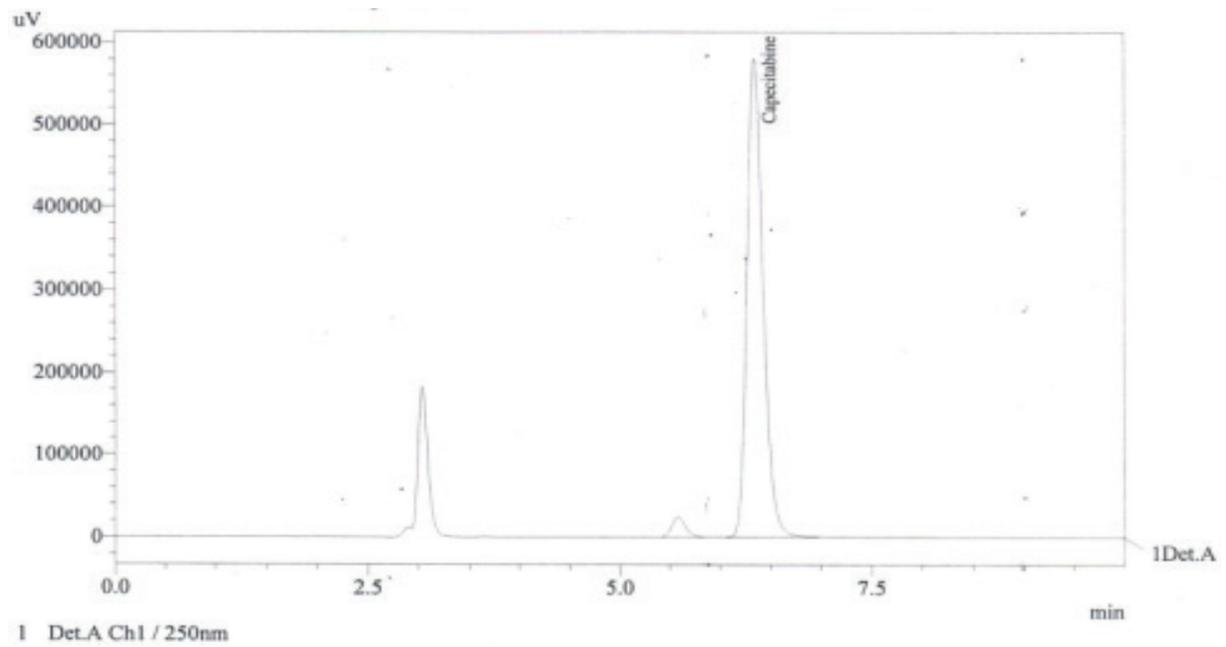
**Figure 3.** Chromatogram for specificity in 0.1M HCl
