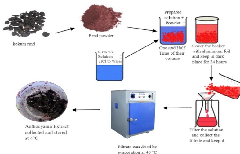
Figure 5: Schematic diagram for extraction of anthocyanin.
