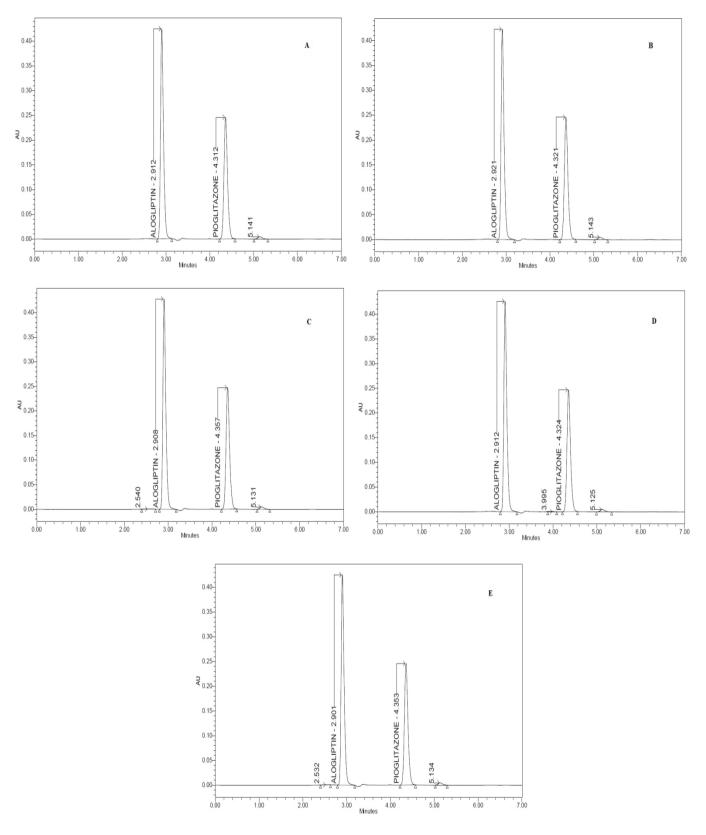
Figure 4. Chromatogram of tablet sample (A) Treated with 0.1 N HCl (B) Treated with 0.1 N NaOH (C) Treated with 30% H<sub>2</sub>O<sub>2</sub> (D) Exposed to 105°C (E) Exposed to sunlight
