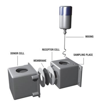
FIGURE 2. The schematic representation of fluid/fluid diffusion cell.
