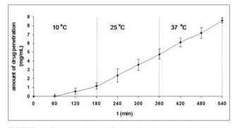
FIGURE 5. The penetration of Sodium Salicylate through cellulose nitrate membrane without COC
